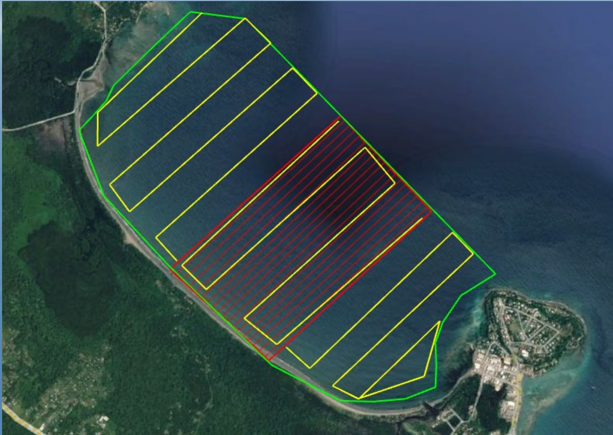
Wewak Proposed Port Site. The 50-meter pitch (red) and the 300-meter pitch (yellow)
